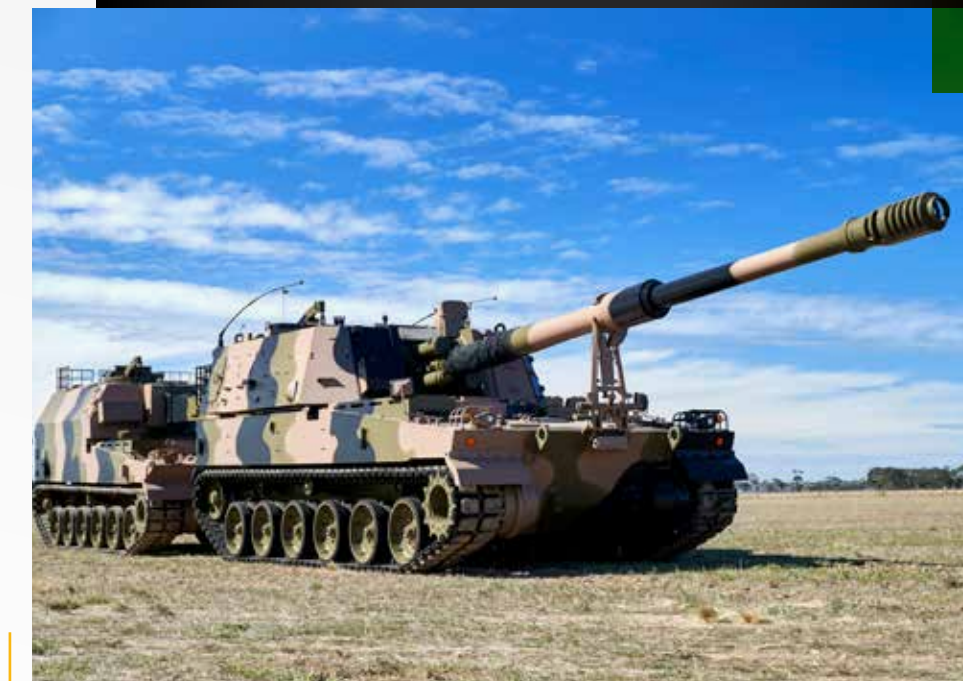
Huntsman AS9 Self-Propelled Howitzer (front) and AS10 Armoured Artillery Resupply Vehicle (rear)
