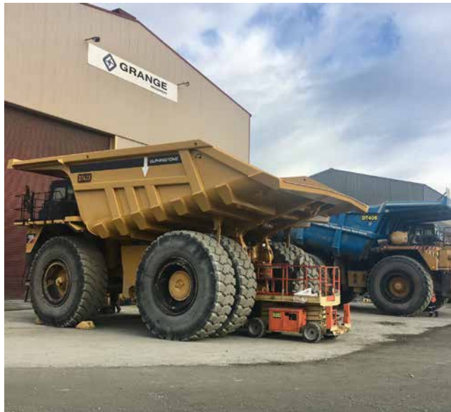
▲ Safely on site, and mounted to the 789D chassis.
